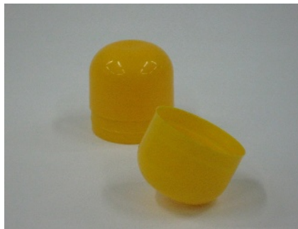
Figure A.5 — Example of non-complying cylindrical shaped packaging with rounded ends
